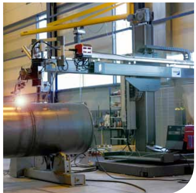
MAG welding with PEMA MD column & boom
