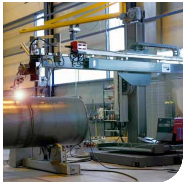
MAG welding with PEMA MD column & boom
