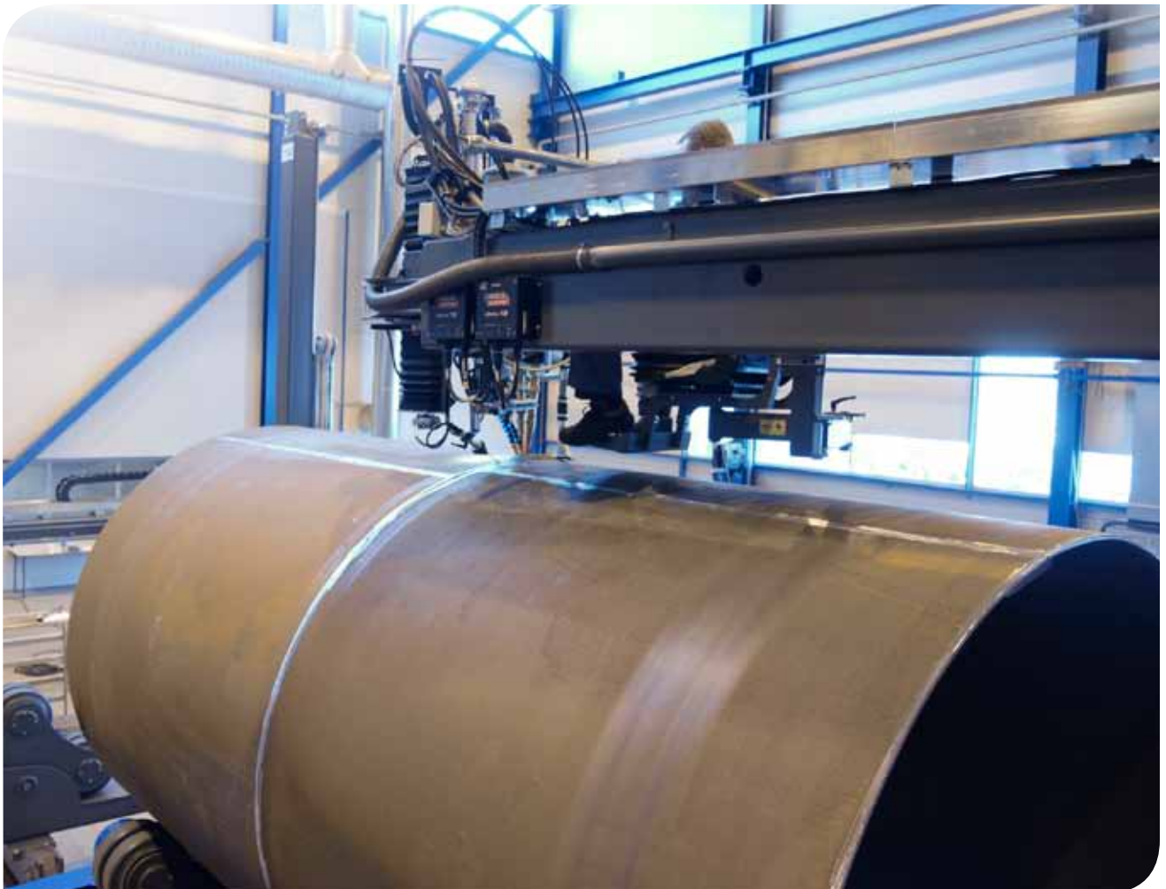
Welding with PEMA column & boom and rollerbeds
